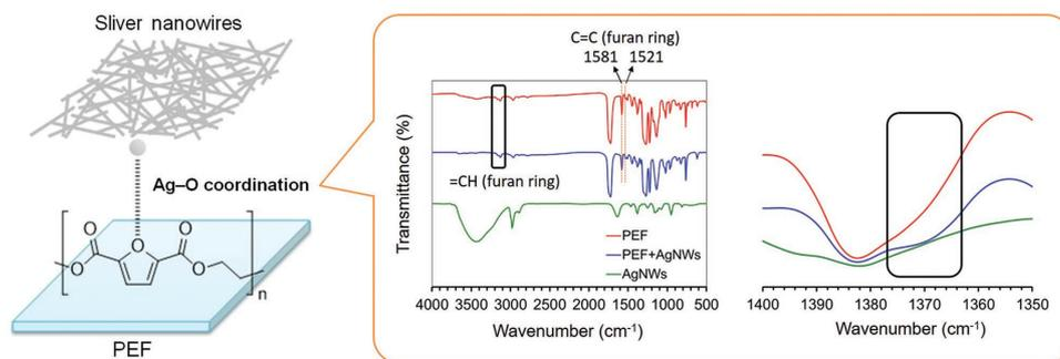
**Figure 1.** Schematic illustration and FT-IR spectra of the PEF substrate, PEF/Ag NWs conductive film, and Ag NWs.
