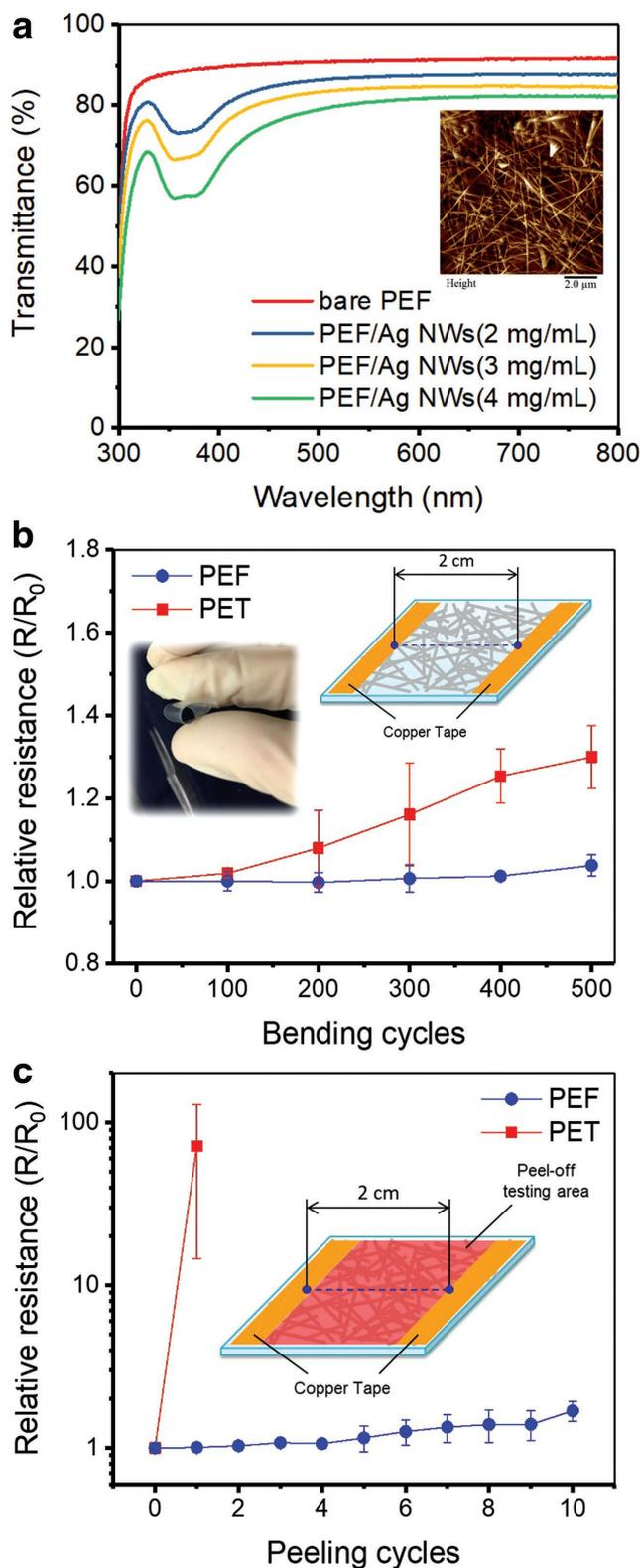
**Figure 2.** a) The transmittance spectra of the PEF substrate and the studied Ag NWs/PEF conductive films with different thickness of Ag NWs. Comparison of the electrical resistance of both PET/Ag NWs and PEF/Ag NWs conductive films as a function of b) bending cycles and c) tape-peeling cycles.
