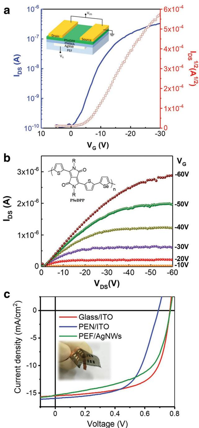
**Figure 3.** a) The transfer and b) output characteristics of a polymer FET using the PEF/Ag NWs conductive film as the bottom gate electrode and substrate (see insert). In (a), a constant  $V_d$  of -60 V is applied. c) The  $J-V$  curves of the inverted organic solar cells using different bottom electrodes, including glass/ITO, PEN/ITO, and PEF/Ag NWs substrates.
